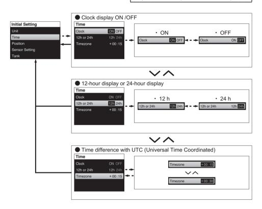
If the gauge is not connected to a GPS module, "--:--" will be displayed. Press the  $\checkmark$  or  $\land$  button briefly to change the time by 15 minutes. If you press and hold the  $\checkmark$  or  $\land$  button, the time will be changed in 15 minute units continuously.
