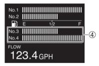
④ Remaining fuel volume (Tank 3) Remaining fuel volume (Tank 4)
